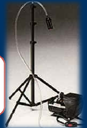
Air clearance check ( < 0.01 f/cc)
